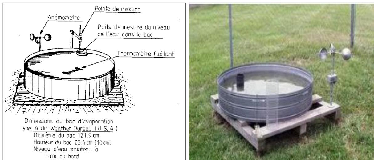
**Figure.6** Bac d'évaporation (classe A) (Source : [https://nanopdf.com/download/medida-de-la-evapotranspiracion\\_pdf](https://nanopdf.com/download/medida-de-la-evapotranspiracion_pdf)).
